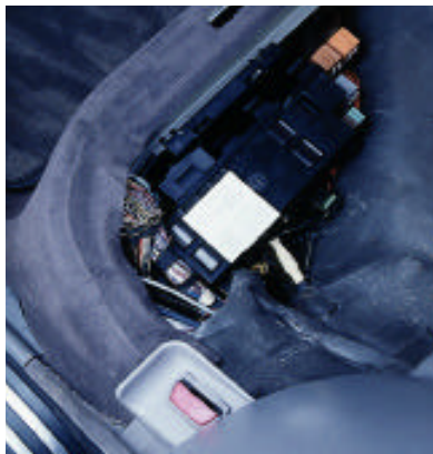
Main relays are under the rear seat so the electronics on these cars are generally reliable.
